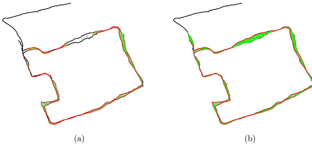
Figure 7.6: Appearance-based loop closure results for the City Center sequence. The positions of the images are plotted as black dots. Wherever an image closes a loop with another image, both are labelled with a red dot and linked with a green line. (a) shows the result of HTMap, while (b) shows the ideal map that should be obtained if all the loops present in the sequence were correctly detected.
