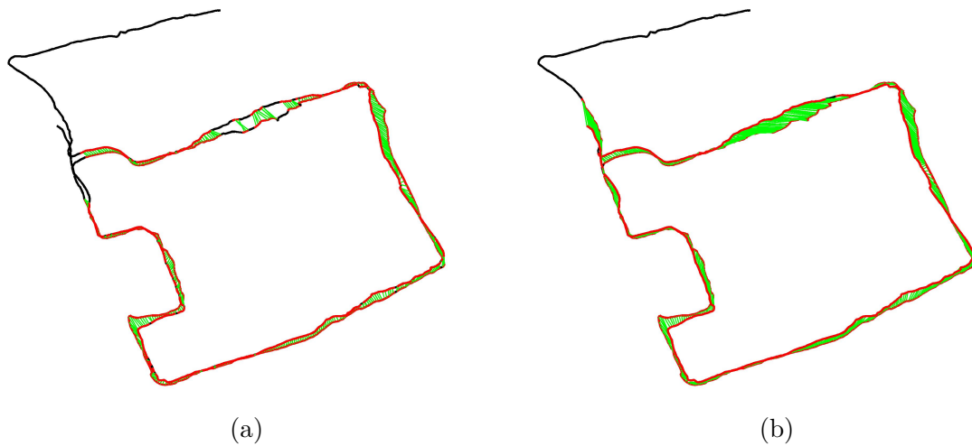
Figure 6.6: Topological map generated for the City Center sequence. The positions of the images are plotted as black dots. Wherever an image closes a loop with another image, both are labelled with a red dot and linked with a green line. (a) shows the result of BINMap, while (b) shows the ideal map that should be obtained if all the loops present in the sequence were correctly detected.
