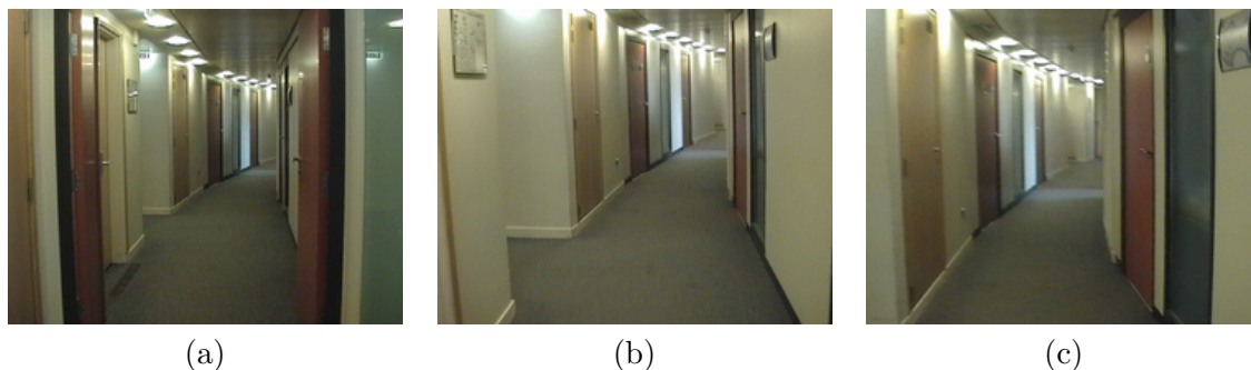
Figure 5.15: Example of adding intermediate nodes in the Lip6Indoor sequence. Images 13 (a) and 86 (c) were added to the map at the first loop. Image 228 (b) was added to the map the next time the camera visited the same place. As can be seen, image 228 is visually in-between the left and the right images.
