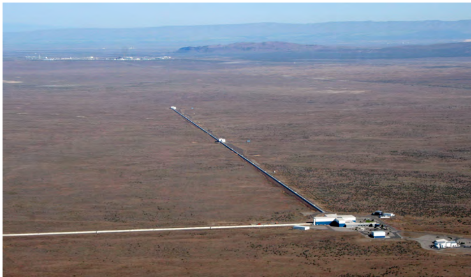
Fig. 1.3: Aerial image of the LIGO Hanford gravitational wave observatory, with 4 km arms. Source: LIGO.
