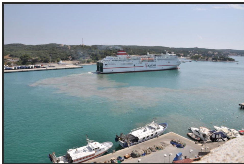
Figure S2.2 A deep-draft vessel manoeuvring in the inner basin of Maó Harbour, and resuspending sediments.
