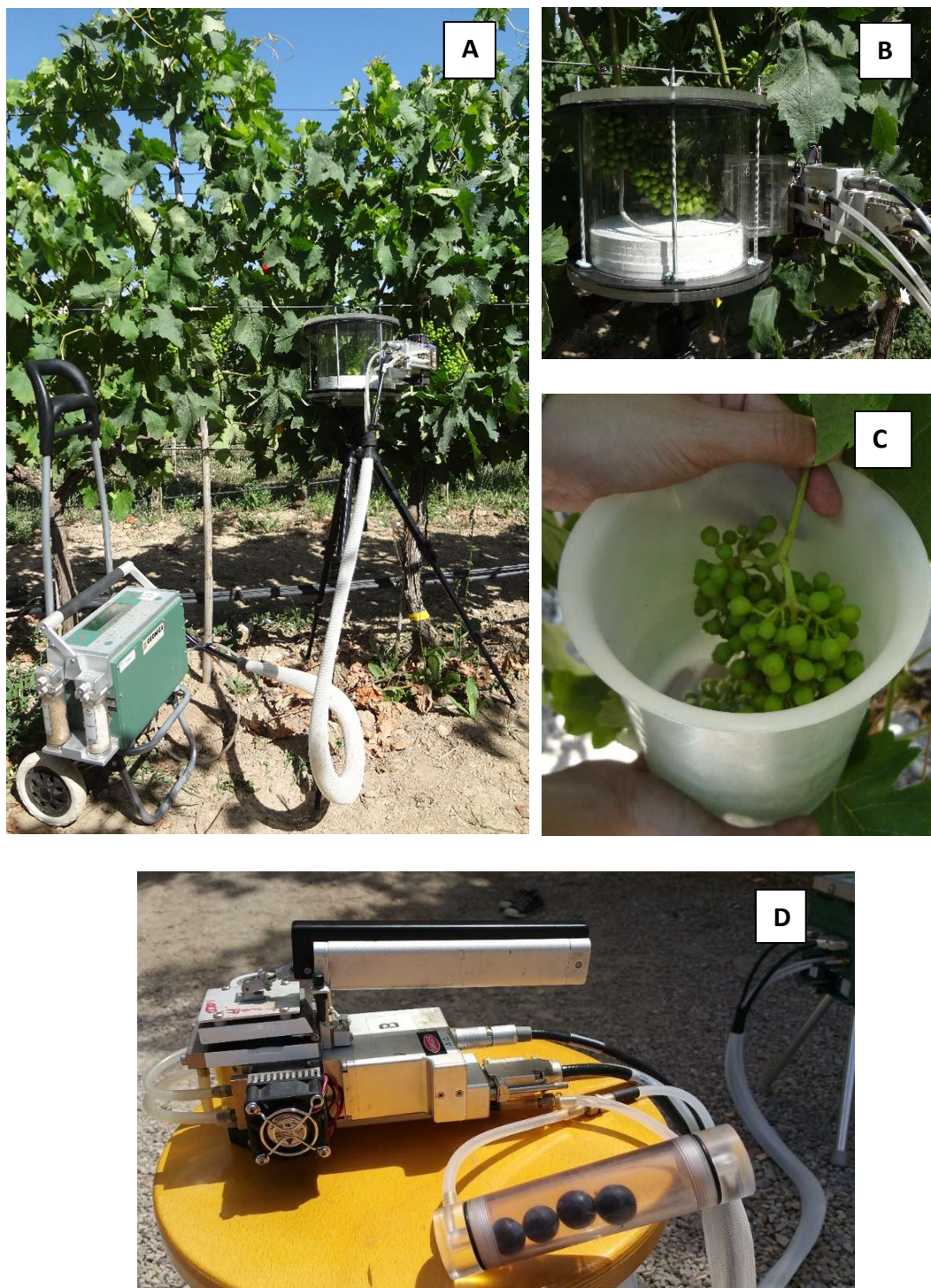
Figure 1 (A) Measurement of whole attached cluster respiration using a fruit respiration chamber connected to a portable gas exchange analyzer (LI-6400). (B) A close up of the fruit chamber with an attached cluster inside. (C) Measurement of the cluster volume using a non-destructive technique. (D) Measurement of detached isolated berries using a specific chamber (LI-6400-89 insect respiration kit) connected to a portable gas exchange analyzer (LI-6400).
