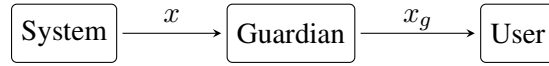
Figure 3.5: Restricting a system’s failure semantics by means of a guardian. The guardian provides the same external states as the system unless it detects that the system’s service is incorrect. When that happens, it produces a service corresponding to a restricted failure mode.
