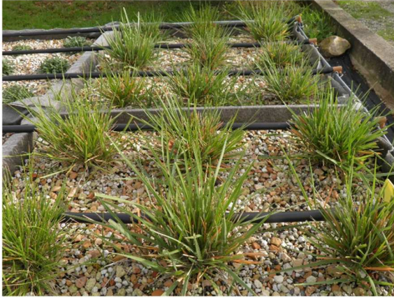
Figure 6.2. A. Experimental metal module covered with Brachypodium phoenicoides at the beginning of experiment (spring 2014), 88% to 94% soil cover. B. Experimental metal module covered with Sedum sediforme at the beginning of experiment (spring 2014), 90% to 94% soil cover.
