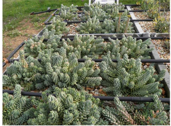
Figure 6.2. A. Experimental metal module covered with Brachypodium phoenicoides at the beginning of experiment (spring 2014), 88% to 94% soil cover. B. Experimental metal module covered with Sedum sediforme at the beginning of experiment (spring 2014), 90% to 94% soil cover.
