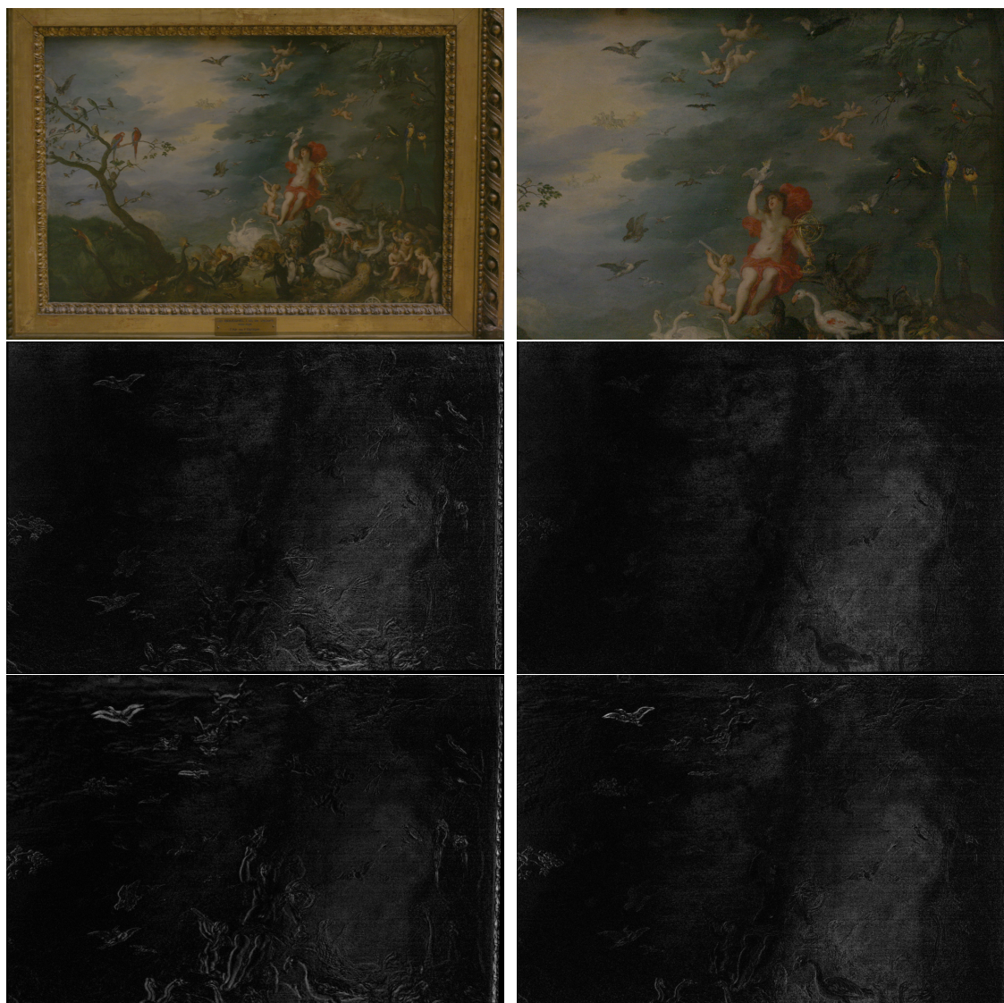
Figure 5.4 – RANSAC (left) and RANSAAC (right) registration results. Dynamic ranges were stretched to highlight differences. Top: input images. Middle: registration difference using input images. Bottom: registration difference by adding measurement noise of \sigma = 10 to the keypoint positions on both images in pixels. Edges due to misalignments can be perceived in the difference image, particularly by using the traditional RANSAC method. Painting: L'Air, ou L'Optique. Jan I BRUEGHEL, 1621. Louvre Museum.
