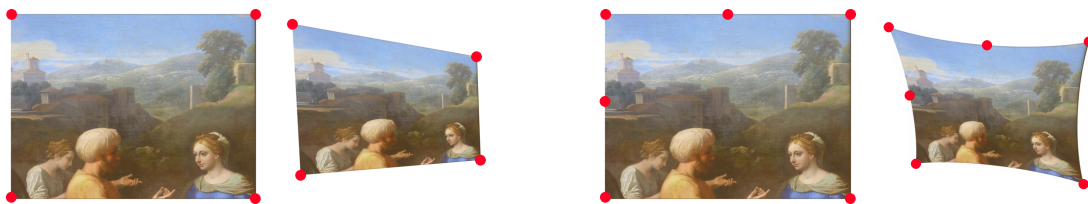
Figure 5.2 – Suggested predefined source points (in red). Left: for homography estimation. Right: for homography + distortion.
