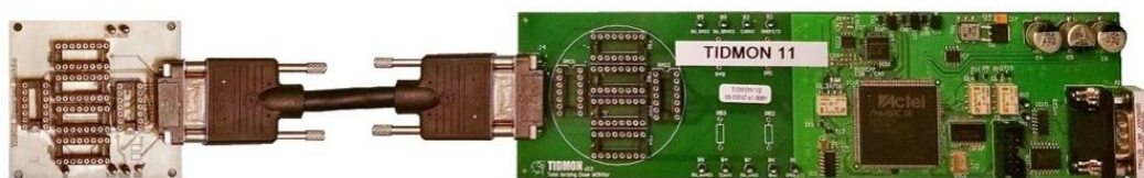
Figure 14. TIDmon system, composed by TIDmon board and deported module
