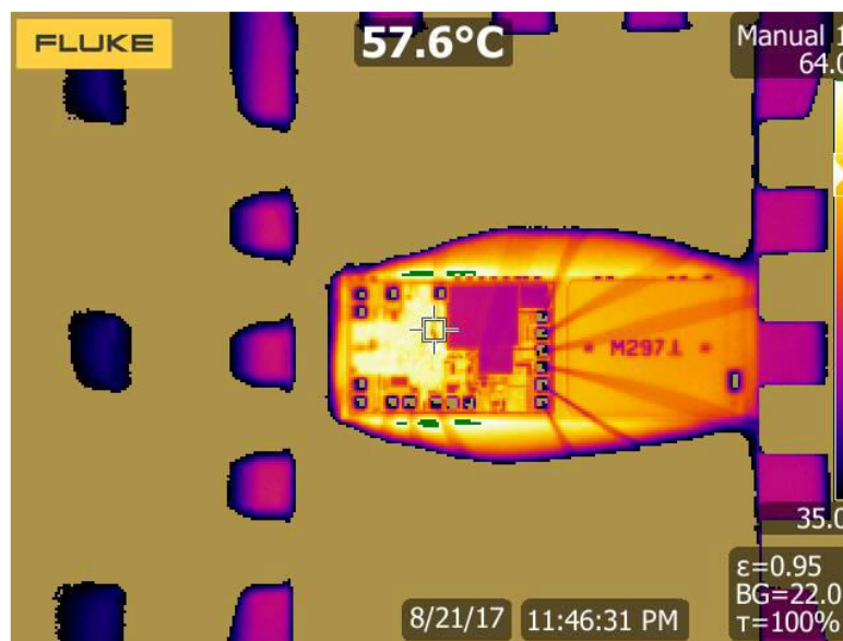
Figure 57. TC974 version 1, thermography experiment, 300 Gy of cumulated TID
