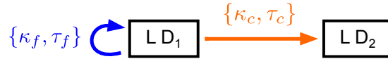
Figure 4.1: Scheme of the open loop coupling configuration studied in detail in section 4.3. This setup is an adaptation, originally by Heilighenthal et al [59], of the Abarbanel’s original setup for delay-coupled systems. The identical synchronization state existed when the coupling and feedback parameters were identical.
