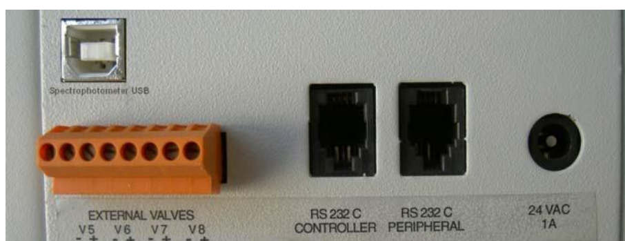
Figure 3.5 Backside connections of a multisyringe pump.
