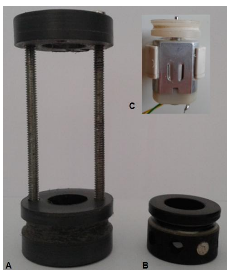
Figure 3.11 A) External device for up multisyringe, B) external device for upside-down multisyringe and C) motor.
