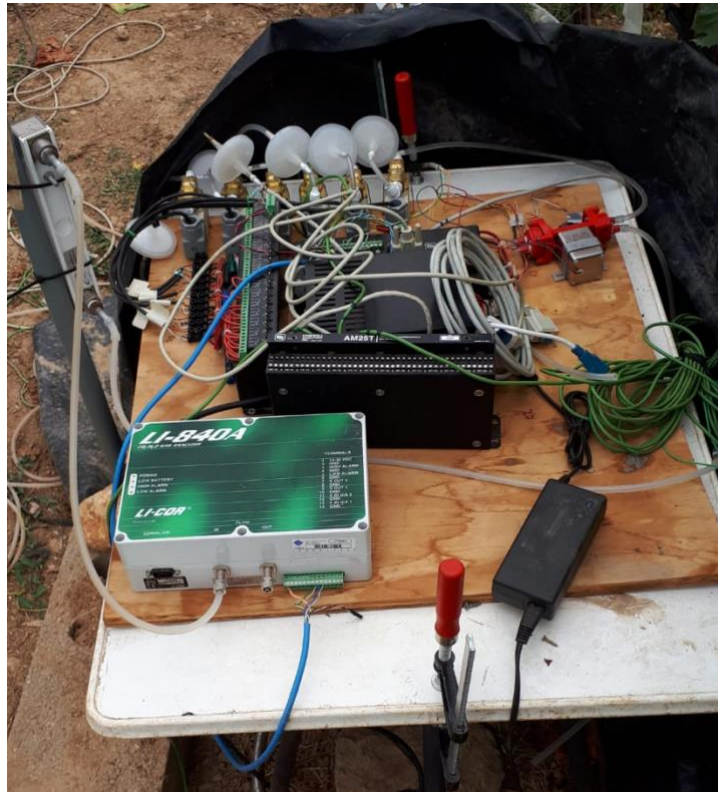
Figure 2. System that controlled and measured all the inputs and outputs of both chambers.
