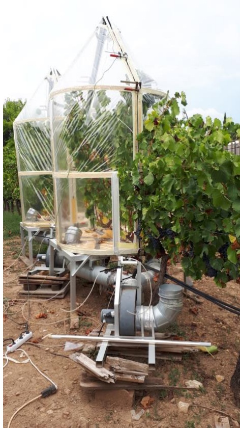
Figure 1. The two whole-plant gas exchange chambers used during the experiment.
