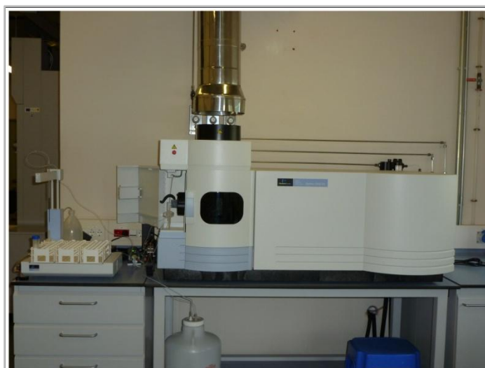
Figure 22. Photograph of the inductively coupled atomic plasma emission spectrometer (ICP-AES Optima 5300DV, PerkinElmer, Massachusetts, USA) used to quantify calcium content.
