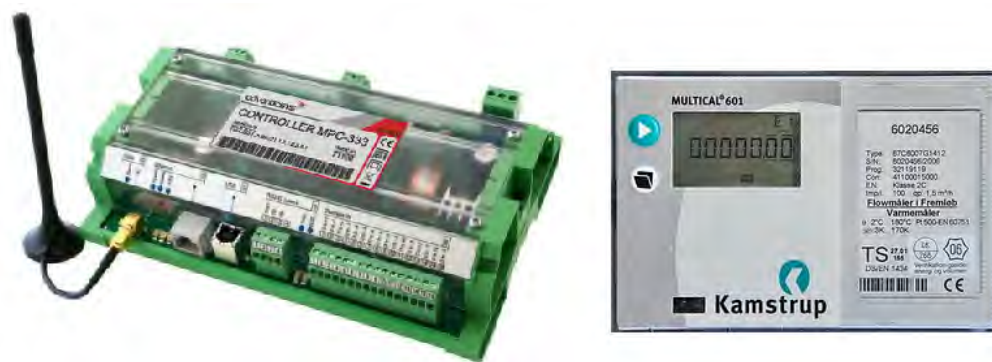
Figure 5.8: Datalogger + Kamstrup Multical 601
