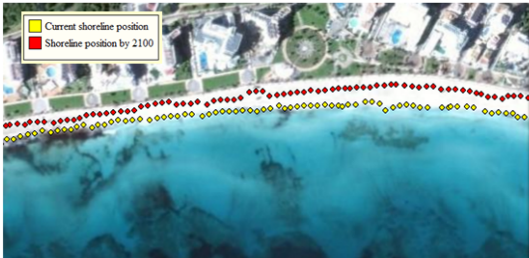
Figure 2.17 Present-day shoreline position (in black) and landward migration (in red) in the worst case scenario (mean sea-level rise under RCP8.5 and extreme wave conditions) by the end of the 21 st century in the Cala Millor beach.
