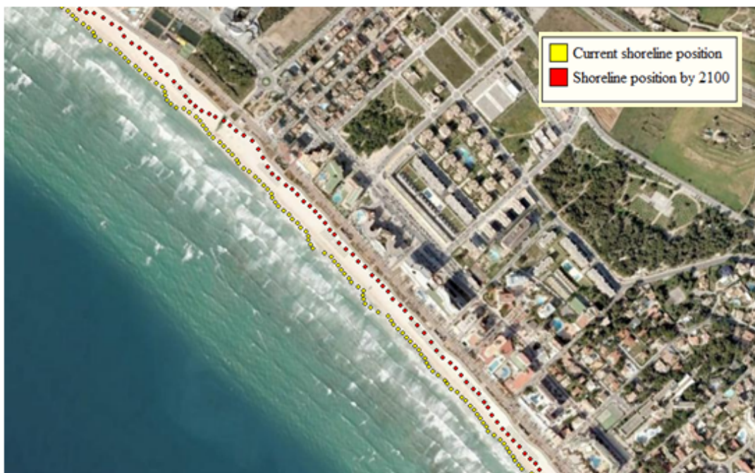
Figure 2.18 Present-day shoreline position (in black) and landward migration (in red) in the worst case scenario (mean sea-level rise under RCP8.5 and extreme wave conditions) by the end of the 21 st century in Playa de Palma.
