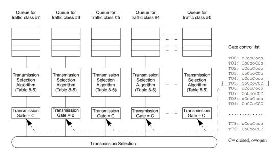
Figure 2.8: Transmission selection with gates [5]
