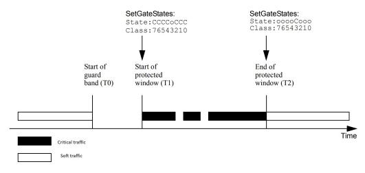
Figure 2.9: Protected window using scheduled traffic [5]
