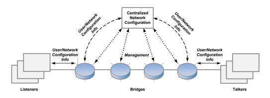
Figure 2.5: Centralised network/distributed user model [4]
