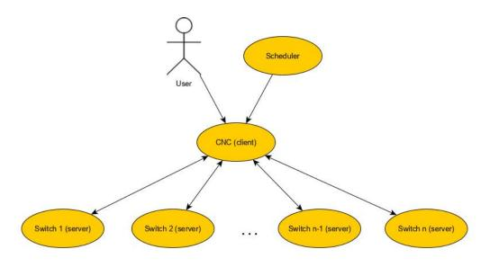
Figure 4.8: Centralised network/distributed used model depicted in our system
