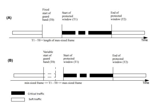
Figure 2.7: Establishing a protected window [5]
