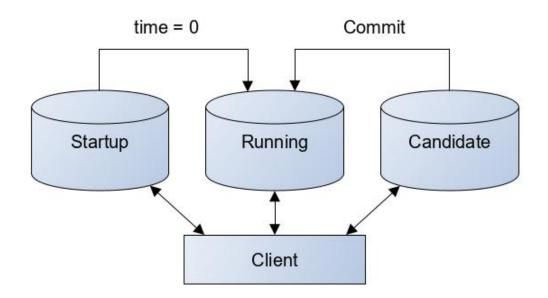
Figure 2.10: NETCONF configurations datastores
