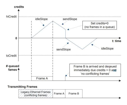
Figure 2.3: Credit-based shaper (CBS) operation [3]
