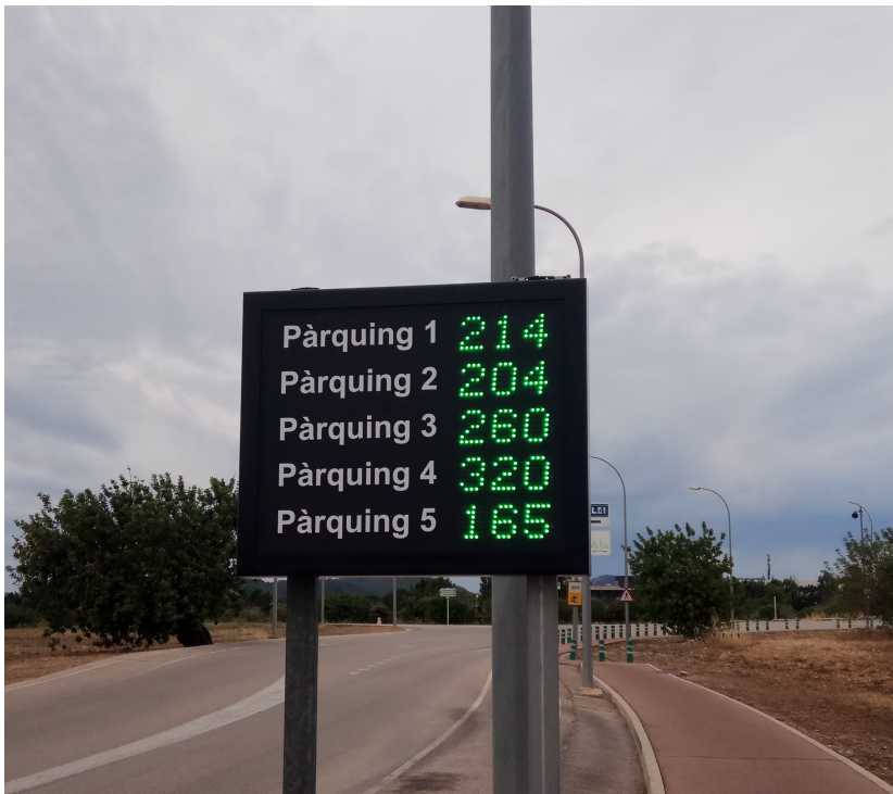
Figure 5.12: 5-line display showing the quantity of free spots in every parking zone.
