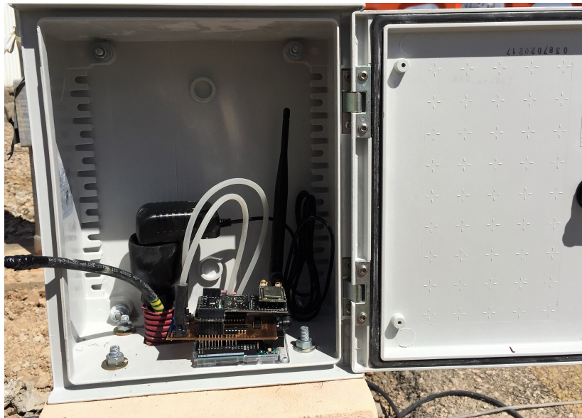
Figure 5.2: The node (S2) is connected to the power source and the pressure tubes.
