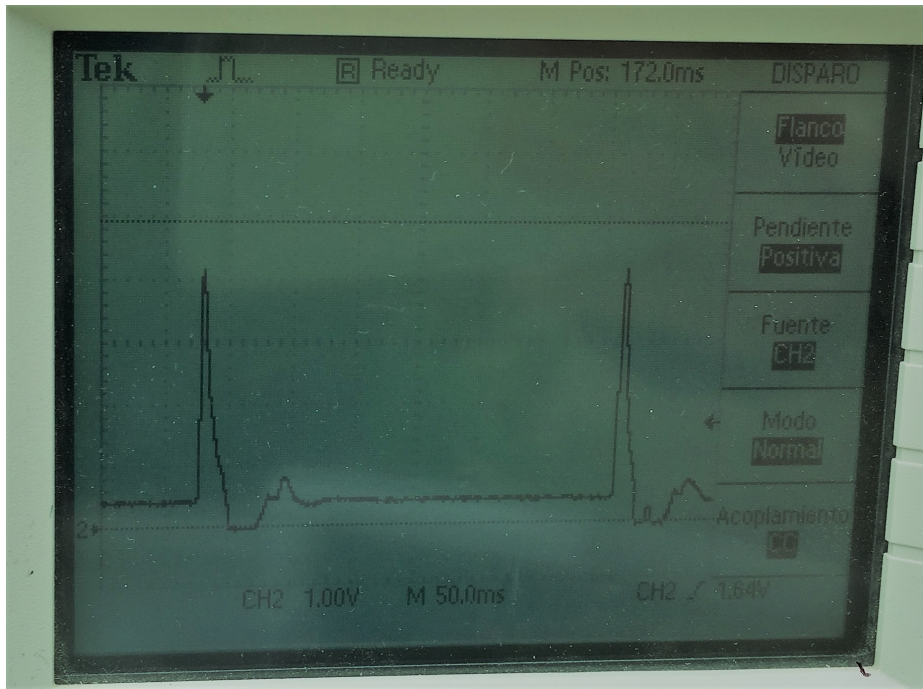
Figure 4.4: Voltage time response caused by a car (vehicle 1) while passing at 29 Km/h
