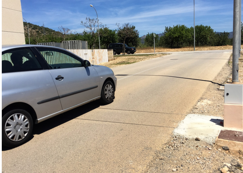
Figure 5.5: The vehicles pass over the tubes disposed on the asphalt.
