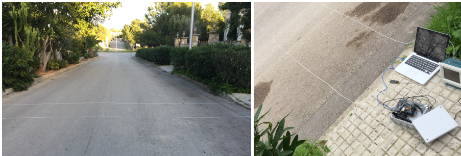
Figure 4.3: Setup for the experiment in a street of Santa Ponsa. For the voltage supply we used the power of PC USB as shown in figure 4.3. The ground of the scope was connected to the ground of the USB.
