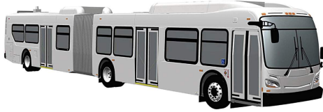
Figure 4.27: Instance of a bus with 3 axis: Excelsior model XB60. If a vehicle has more than two axis it won't fall within our detection mechanism. It will detect one car and a half.
