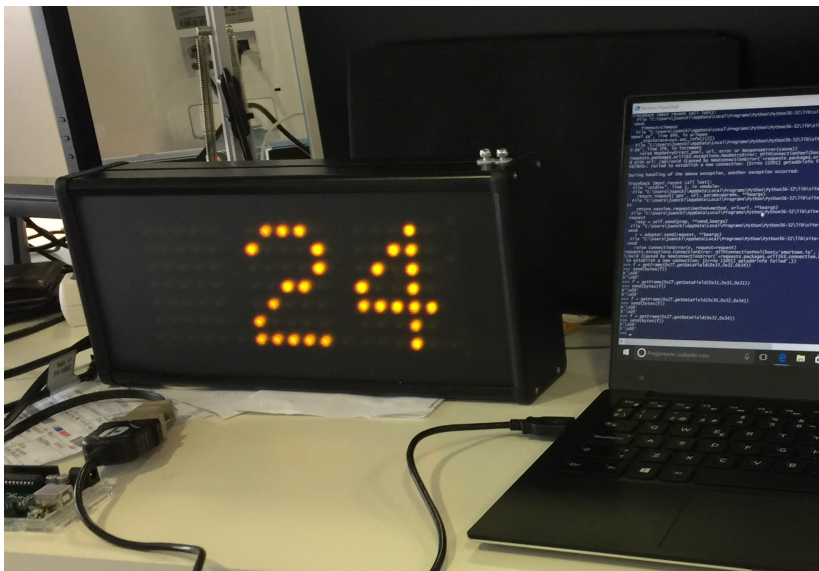
Figure 5.8: Display connected to the laptop's USB via a transceiver USB to RS232. The python script made controls serially the screen.
