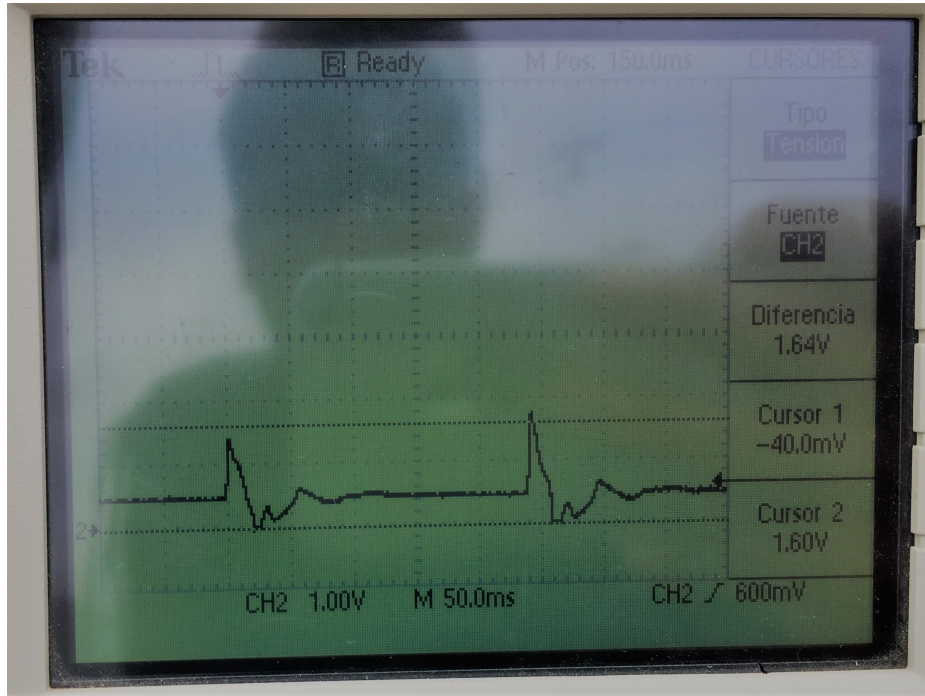
Figure 4.5: Voltage time response caused by a moto (vehicle 3) while passing at 20 Km/h
