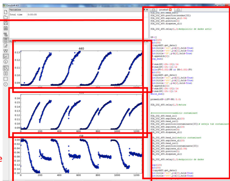
Fig. 2. Screenshot of CocoSof program during unsupervised system execution. The fluidic method is executed in the right column of the screen, the 440 and 490 nm emission intensities are acquired at real time and the GP value is calculated in-situ as seen at the left side of the image.
