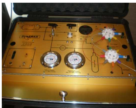
Figure 3.4. Hydraulic Conductance Flow Meter (HCFM-XP).
