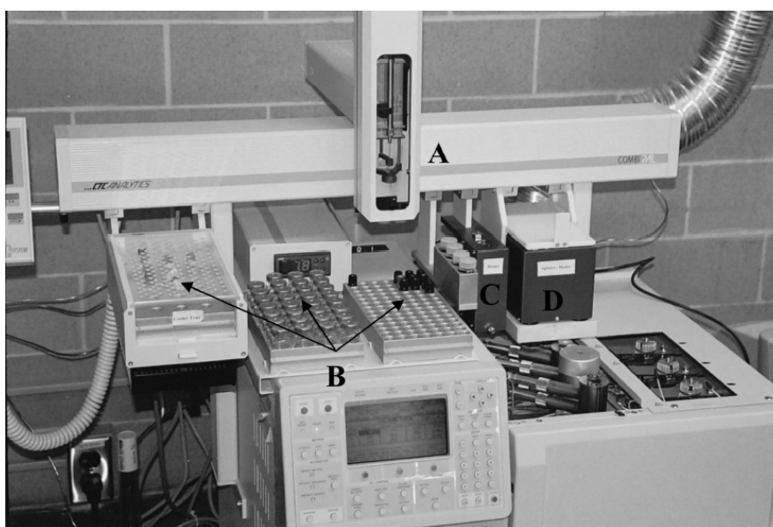
Figure 34. Commercial SPME-GC autosampler (CTC Analytics CombiPAL); A:sample preparation/injection arm, B:sample trays, C:needle heater, D:heater/agitator.
