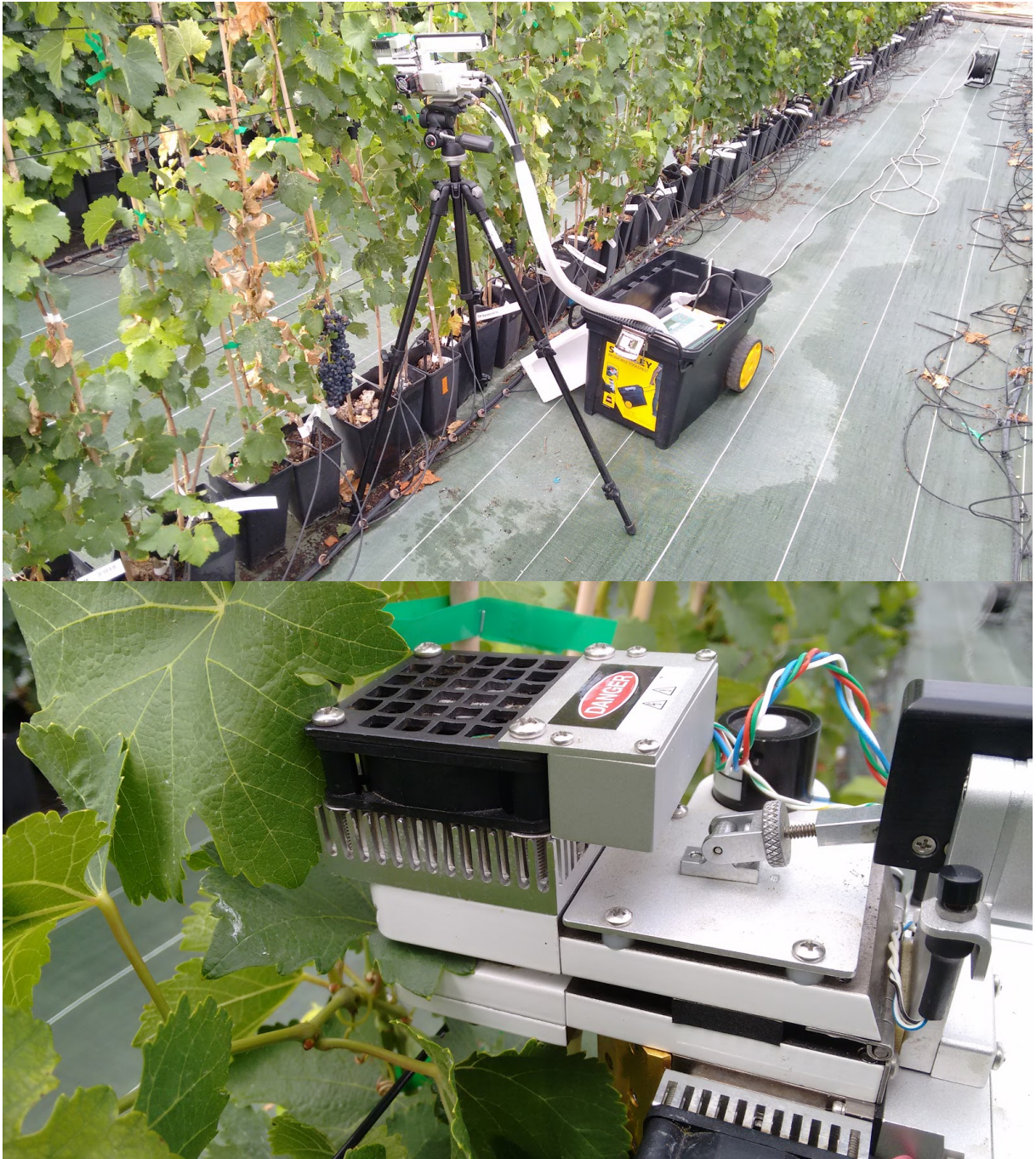
Figure 3. Process of taking leaf gas exchange measurements with an open infrared gas-exchange analyzer during experiment 2.
