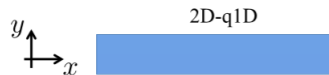
Figure 2.5: Scheme of infinite quasi-one dimensional nanowire along x with y as the transverse dimension. Image taken from [5].
