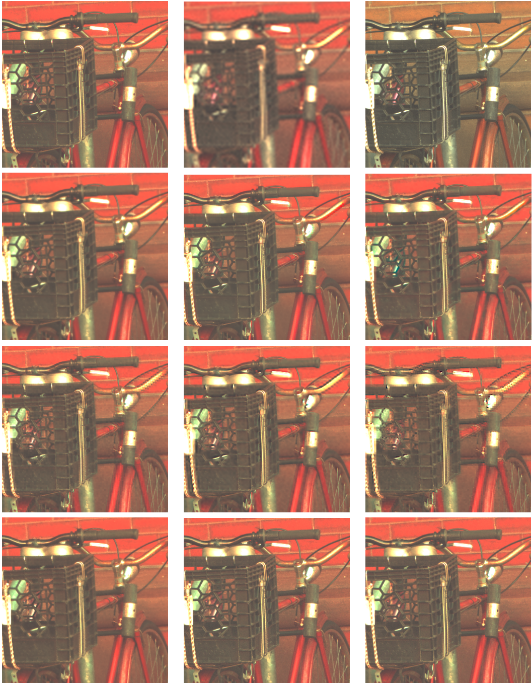
Figure 3.9: Performances of HS-MS fusion with the nonlocal-gradient-based method and comparison with other state of the art methods on Harvard dataset, image "Bicycles" of size 512 \times 512 \times 31 . From top left to bottom. Reference image, HS image, MS image, CNMF, HySure, GSA, SFIMHS, GLPHS, MAPSMM, HMWB, L^2 norm and L^1 .
