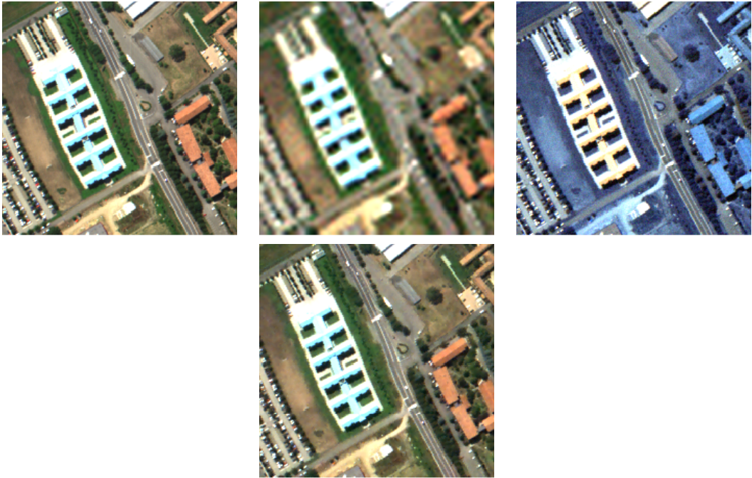
Figure 1.9: Performances of HS-MS fusion with optimal transport on Pavia dataset 256 \times 256 \times 93 . From top left to right. Reference image, HS image, MS image and the result of the proposed method.
