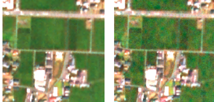
Figure 2.24: Result of fusion on the Chikusei data set. Left: fusion with denoising. Right: fusion without denoising. Both results are in the case where \xi = \xi^{\text{dist}} .
