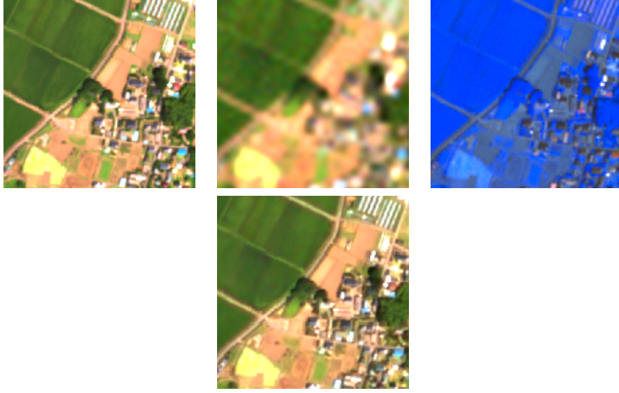
Figure 1.10: Performances of HS-MS fusion with the nonlocal gradient based method on Chikusei dataset 304 \times 304 \times 93 . From top left to right. Reference image, HS image, MS image and the result of the proposed method.
