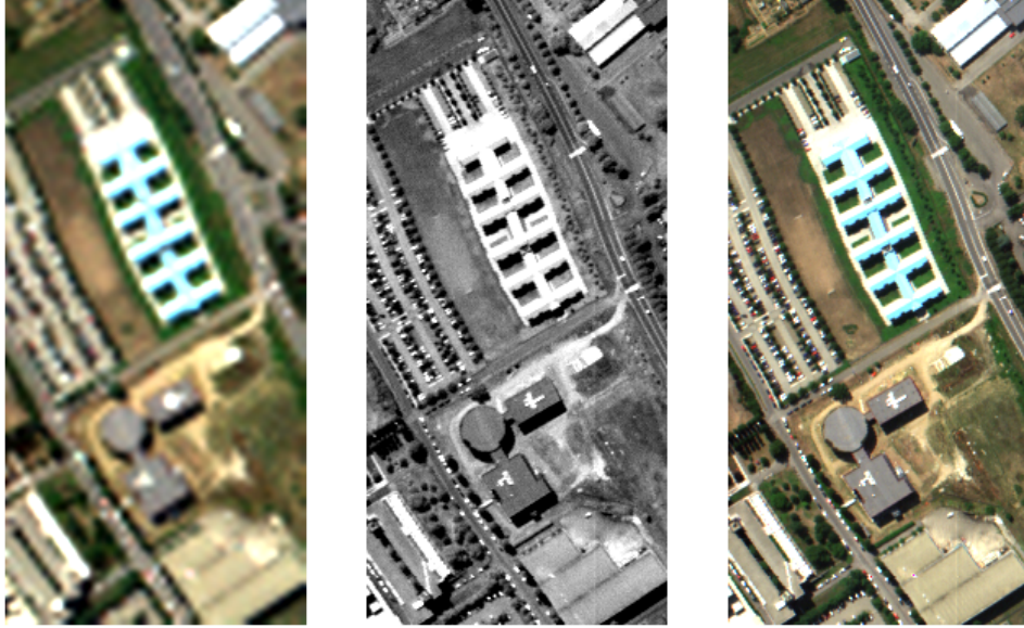
Figure 1.8: (Left) Hyperspectral image (size: 99 \times 46 \times 224 ). (Middle) Panchromatic image (size: 396 \times 184 ). (Right) Target image (size: 396 \times 184 \times 224 )
