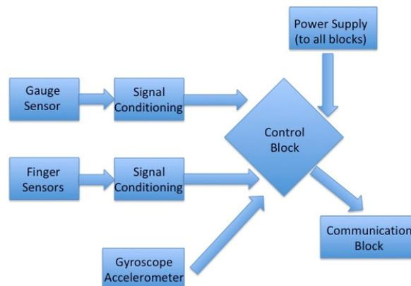
**Figure 2.** Hardware components of the device.
