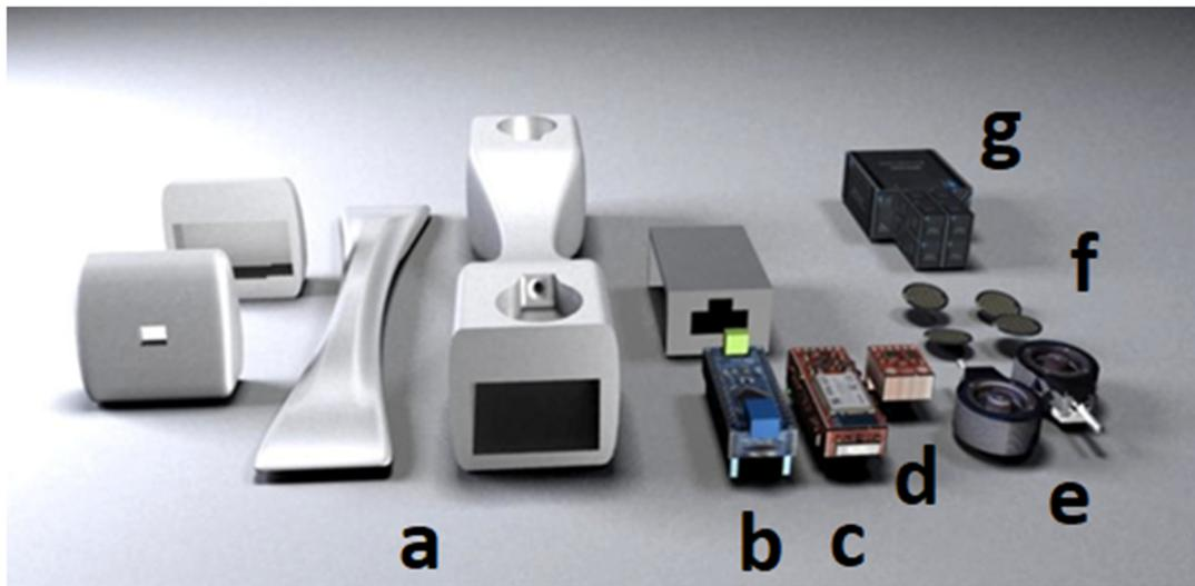
**Figure 1.** Shaders prototype and their components: (a) controller case, (b) Arduino, (c) Instrumentation Amplifier (AD627), (d) IMU sensor, (e) force sensors, (f) Interlink FSR sensor, and (g) battery.
