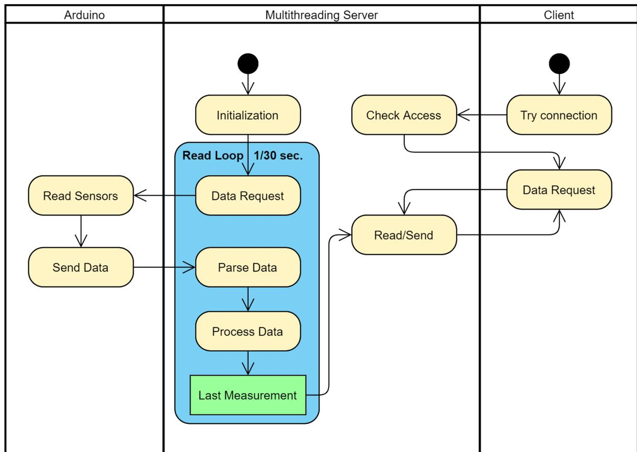
**Figure 5.** UML communication diagram. Server is running in multithread. Main thread communicates with Arduino, and one thread runs for each client.
