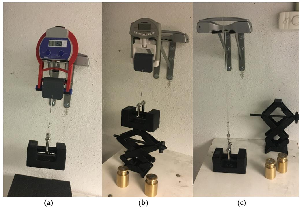
**Figure 12.** Dynamometers cargo system. (a) Takei 5101 TKK, (b) Constant 14192-709E, (c) hand grip device UIB
