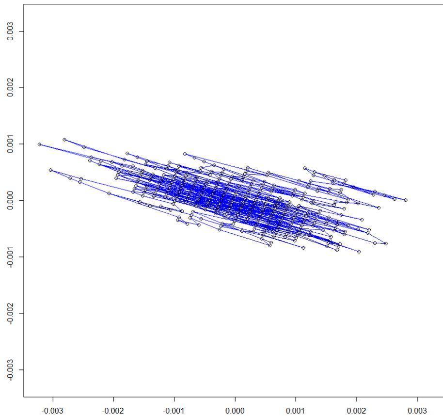
**Figure 9.** Stability measurement for orientation yaw =  $-176.8162$ , pitch =  $-17.0508$  and roll =  $109.87212$ . The difference between orientations has been measured by the L2 norm of the projection of the orientation on the unit sphere. The maximum error obtained is  $1.135321 \times 10^{-5}$ , which is equivalent to a maximum error in degrees of  $0.1930557$  in degrees.
