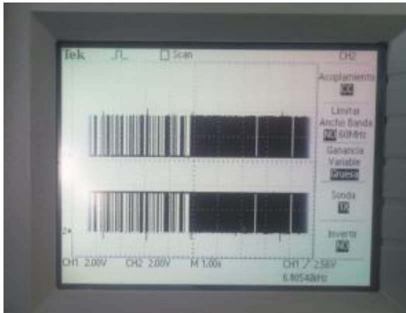
Figure 3.10: Snapshot of the oscilloscope showing the control signals of the analog switch. The upper signal is \Phi_1 , while \Phi_2 is the lower signal. Notice that both signals are complementary and non-overlapping.
