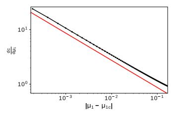
FIG. 6. Scaling of the derivative of the velocity of the TP with respect to  $\mu_1$  in the proximity of the SNSL. The expected theoretical scaling is shown in red for comparison.
