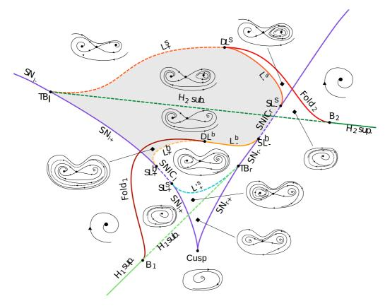
FIG. 1. Schematic phase diagram for the  $\mu_1$ ,  $\mu_2$  plane for fixed  $\nu=1$ , b=2.4 parameters of equation (2). The lines represent the bifurcations that separate the parameter space in qualitative different behavior of the system. The dots mark the codimension-two points. The diagrams show a schematic representation of the phase portrait in the different regions. Gray area marks the excitability region.
