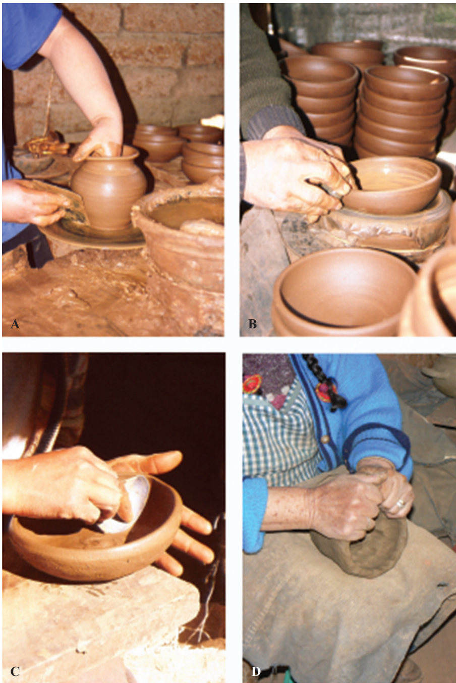
Figure 7. Handmade and pottery wheel technical gestures. A – building pot with potter’s wheel and tool. B – Surface treatments with potter’s wheel and river pebble. C – Traditional hand-made surface treatments. D – Traditional hand-made building pot. Author’s photograph, 1999–2007.
