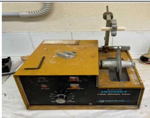
Sierra Isomet Low Speed Saw
