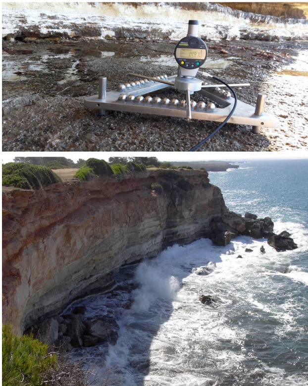
Fig. 2 Traversing-micro-erosion meter used in this study and the supratidal bolt site characterized at s'Alavern shore platform
