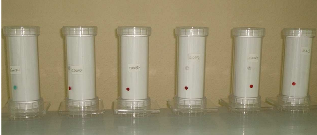
Figure 1. WHO test used for the assessment of Culicoides sensitivity to deltamethrin with five different concentrations of insecticide (red dots) plus the control test (green dot)
