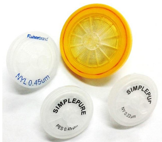
Figure 1.6. Examples of syringe filters with different pore sizes (0.22 and 0.45 \mu\text{m} ), filtering surfaces 15 and 25 cm), and chemistries (Nylon, Polyethersulphone (PES), Polyvinylidene fluoride (PVDF))
