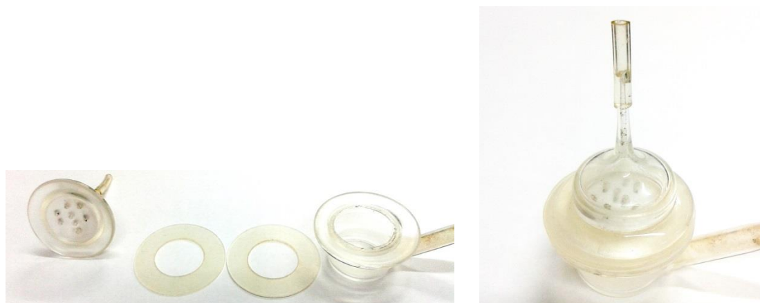
Figure 1.11. Disassembled and closed stirred flow cell showing the upper and bottom glass parts, as well as PDMS washers for holding the commercial filter membrane in place.
