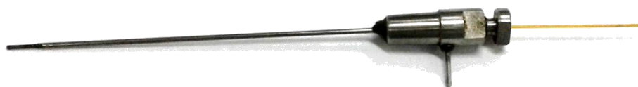
Figure 1.7. Commercial concentric dialysis probe showing the central body with a metal outlet and a GC capillary column as inner cannula serving as perfusate inlet. Note the step at the left of the probe, used for fixing the dialytic membrane. More details on chapter 6.
