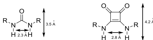
Figure 27. Comparison of the size and internitrogen distances for urea and squaramide moieties.
