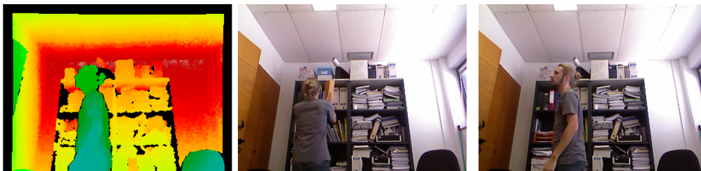
Fig. 4.15: Depth camouflage sequence. Left frame depicts an example of depth frame for this sequence. Two next frames depict the start and the end of the sequence.
